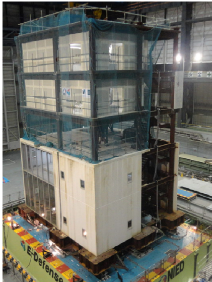
5-Storey Steel Frame Building [1] Shake Table Testing
